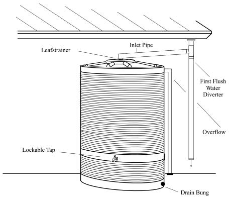
Standard Fittings Include Leafstrainer, Lockable Tap, Mosquito Proof Overflow and Drain Bung.
