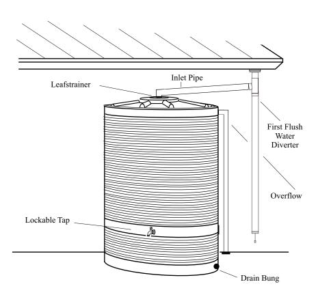
Standard Fittings Include Leafstrainer, Lockable Tap, Mosquito Proof Overflow and Drain Bung.
